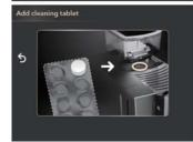
Open the coffee powder container lid, add the cleaning tablet. Close the coffee powder container lid and press "MENU/OK" for confirming.
