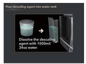
Take a bag of decalcifier and sufficiently dissolves it in clean water, then put this mixed liquid to the water tank, and reinstall the water tank to coffee machine
